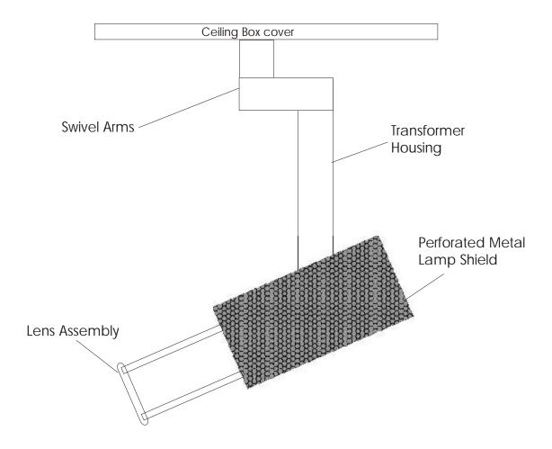
Changing Lamp: Remove Power and let fixture cool down. Carefully slide lamp shield back and rotate to unhook shield from inner rings. Unplug lamp socket. Loosen lamp rim screws and remove lamp. Reverse process to install lamp.
